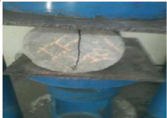
Fig 10. Cylinder Specimen after Failure
