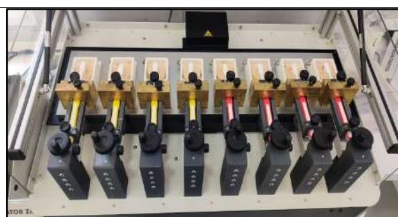
Figure 2: Composite resin samples subjected to brushing simulator
