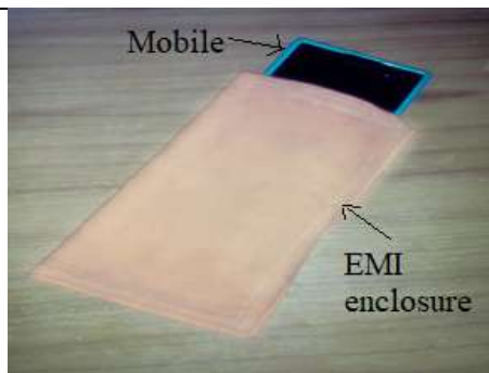
Figure 3. Proposed EMI shielding enclosure designed for Mobile.
