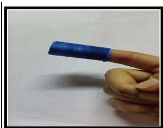
Fig 1: Detection using colour paper attached to fingertip.
