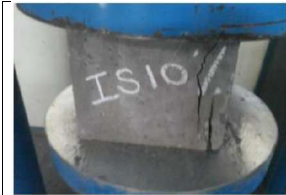
Fig 9. Cube specimen after failure
