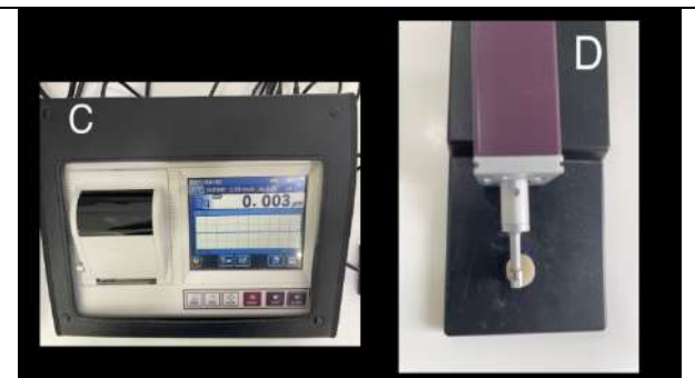
Figure C and D: Stylus Profilometer for surface roughness analysis.
